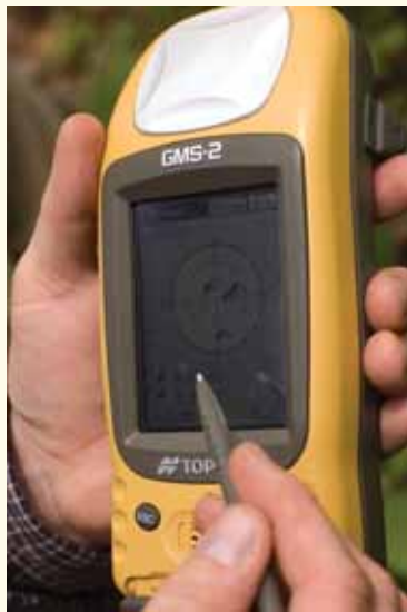
↑ Using a Topcon GMS-2 receiver with camera, points and attributes were entered to populate a GIS database for the trail
